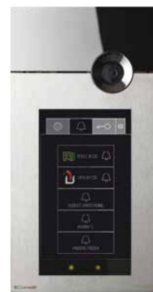
INTERCOM SYSTEM – OUTSIDE COMELIT, digital communication unit with register of names and apartment numbers
